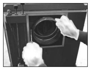
**Figure 8.7** Install the inner collar and outer flue collar on the rear of the appliance.
